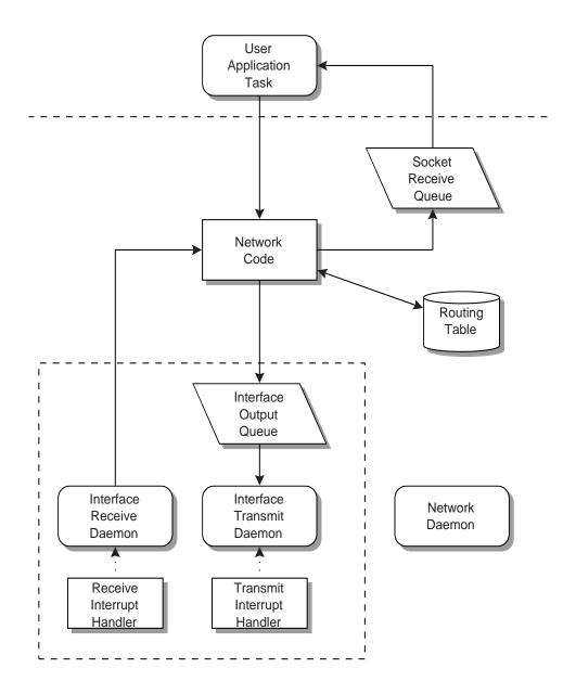
The transmit task for each network interface is normally blocked waiting for a packet to arrive in the transmit queue. Once a packet arrives, the transmit task may block waiting for an event from the transmit interrupt handler. The transmit interrupt handler sends an RTEMS event to the transmit task to indicate that transmit hardware resources have become available.
