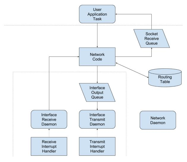
The transmit task for each network interface is normally blocked waiting for a packet to arrive in the transmit queue. Once a packet arrives, the transmit task may block waiting for an event from the transmit interrupt handler. The transmit interrupt handler sends an RTEMS event to the transmit task to indicate that transmit hardware resources have become available.
