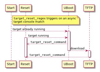
Fig. 11.8: Target Reset Filter Trigger
