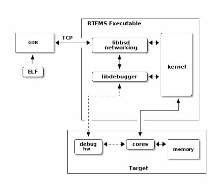
Fig. 10.4: Libdebugger Executable Debugging
