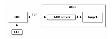
Fig. 10.2: QEMU Executable Debugging
