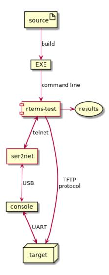
Fig. 11.5: RTEMS Tester using TFTP and U-Boot.
