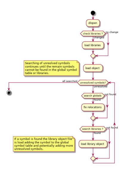
Fig. 9.4: Loading Executable Object Files
