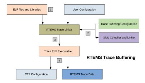
linker uses the target compiler and linker to create the trace enabled application executable. It wraps the functions defined in the user's configuration with code that prints the entry with arguments and exit and return value if any. The trace wrapper code is compiled with the target compiler and the resulting ELF object file is added to the standard link command line used to link the application and the application is relinked using the wrapping option of the GNU linker.
