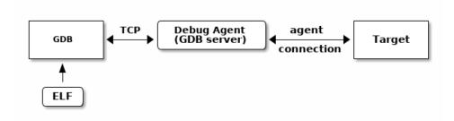
Fig. 10.1: Embedded Executable Debugging
