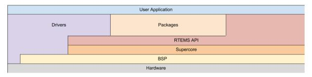
RTEMS targets are grouped by architectures and within an architecture there are a number of Board Support Packages or BPSs. An architecture is a specific class or family of processors and can be large such as ARM or specific such as the NIOS-II or Microblaze.
