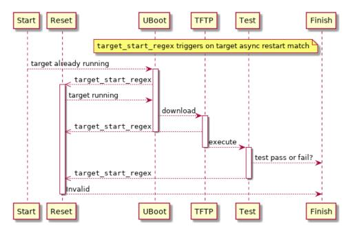
Fig. 11.7: Target Start Filter Trigger
