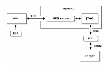
Fig. 10.3: OpenOCD JTAG Executable Debugging
