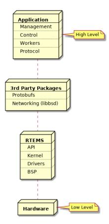
Fig. 9.1: Vertical Software Stack
