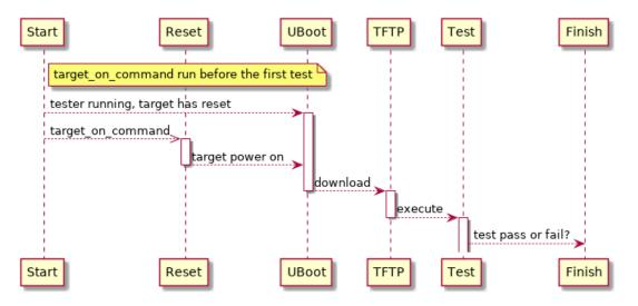
Fig. 11.6: Test Pass and Fail Sequences
