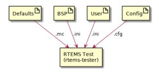
Fig. 11.1: RTEMS Tester and Run Configuration Files
