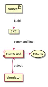
Fig. 11.3: RTEMS Tester Simulation
