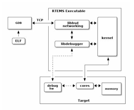
Fig. 10.4: Libdebugger Executable Debugging
