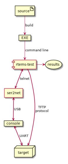
Fig. 11.5: RTEMS Tester using TFTP and U-Boot.
