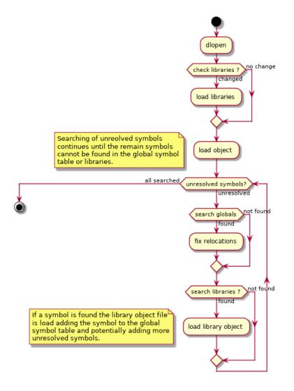
Fig. 9.4: Loading Executable Object Files
