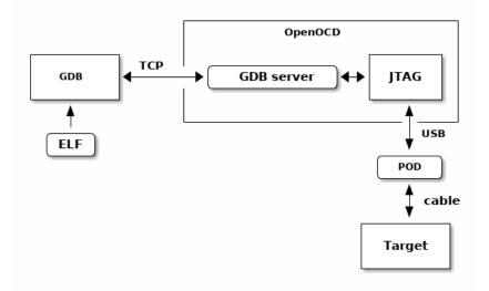
Fig. 10.3: OpenOCD JTAG Executable Debugging
