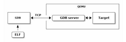
Fig. 10.2: QEMU Executable Debugging
