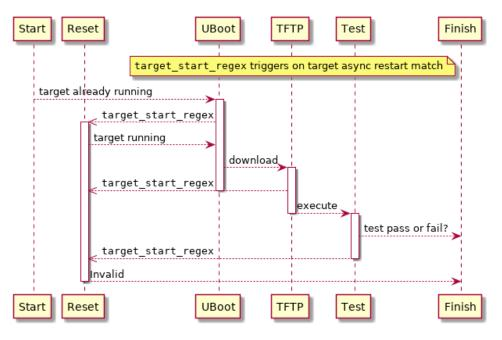
Fig. 11.7: Target Start Filter Trigger
