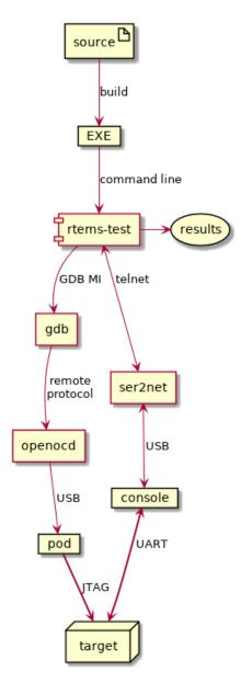
Fig. 11.4: RTEMS Tester using GDB and JTAG
