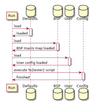
Fig. 11.2: RTEMS Tester and Run Configuration Load and Execute Sequence
