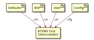
Fig. 11.1: RTEMS Tester and Run Configuration Files
