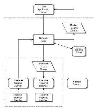
The transmit task for each network interface is normally blocked waiting for a packet to arrive in the transmit queue. Once a packet arrives, the transmit task may block waiting for an event from the transmit interrupt handler. The transmit interrupt handler sends an RTEMS event to the transmit task to indicate that transmit hardware resources have become available.
