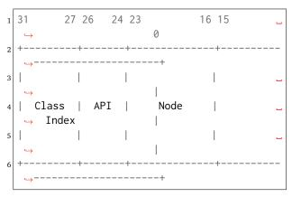
The most significant five bits are the object class. The next three bits indicate the API to which the object class belongs. The next eight bits (16-23) are the number of the node on which this object was created. The node number is always one (1) in a single processor system. The least significant sixteen bits form an identifier within a particular object type. This identifier, called the object index, ranges in value from 1 to the maximum number of objects configured for this object type.
