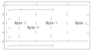
Conversely, processors which place the most significant byte at the smallest address are classified as big endian processors. Big endian byte-ordering is shown below:
