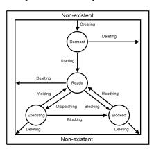
A task occupies the blocked state whenever it is unable to be scheduled to run. A running task may block itself or be blocked by other tasks in the system. The running task blocks itself through voluntary operations that cause the task to wait. The only way a task can block a task other than itself is with the rtems\_task\_suspend directive. A task enters the blocked state due to any of the following conditions:
