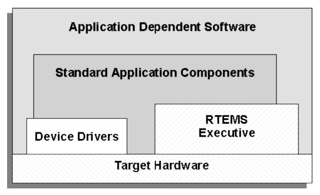
The RTEMS I/O interface manager provides an efficient tool for incorporating these hardware dependencies into the system while simultaneously providing a general mechanism to the application code that accesses them. A well designed real-time system can benefit from this architecture by building a rich library of standard application components which can be used repeatedly in other real-time projects.
