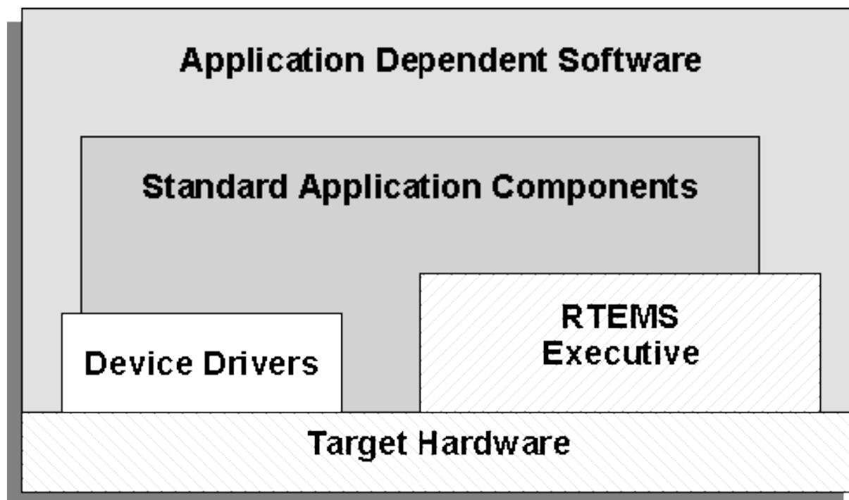
The RTEMS I/O interface manager provides an efficient tool for incorporating these hardware dependencies into the system while simultaneously providing a general mechanism to the application code that accesses them. A well designed real-time system can benefit from this architecture by building a rich library of standard application components which can be used repeatedly in other real-time projects.
