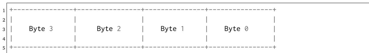
Conversely, processors which place the most significant byte at the smallest address are classified as big endian processors. Big endian byte-ordering is shown below:
