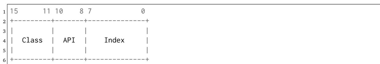
The sixteen-bit format is designed to be as similar as possible to the thirty-two bit format. The differences are limited to the elimination of the node field and reduction of the index field from sixteen-bits to 8-bits. Thus the sixteen bit format only supports up to 255 object instances per API/Class combination and single processor systems. As this format is typically utilized by sixteen-bit processors with limited address space, this is more than enough object instances.
