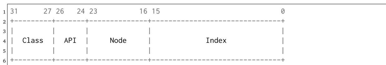
The most significant five bits are the object class. The next three bits indicate the API to which the object class belongs. The next eight bits (16-23) are the number of the node on which this object was created. The node number is always one (1) in a single processor system. The least significant sixteen bits form an identifier within a particular object type. This identifier, called the object index, ranges in value from 1 to the maximum number of objects configured for this object type.
